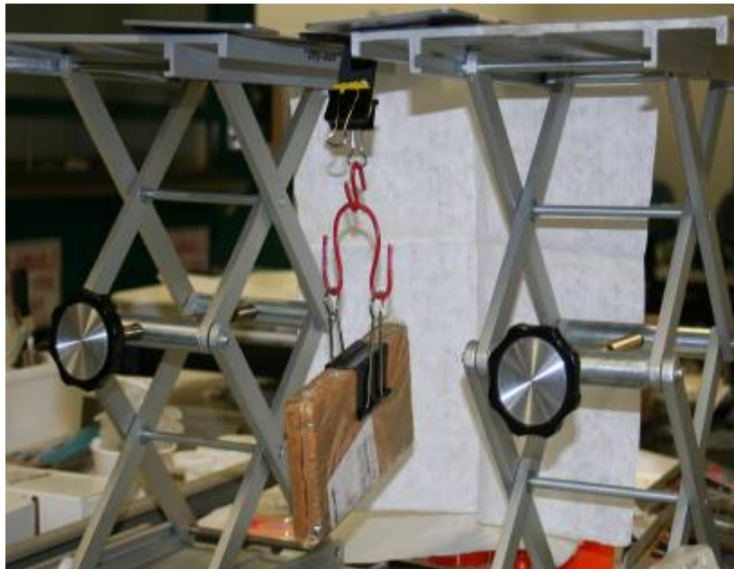
Figure 2. Basic strip adhesion setup for MMM-A-121.
