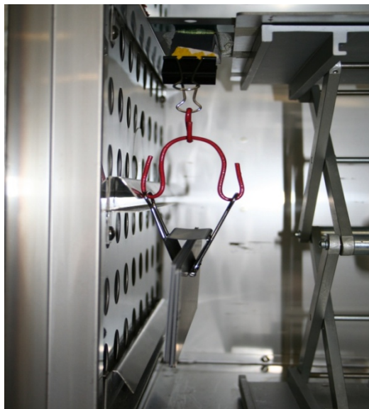
Figure 5. Strip adhesion test in 60 °C oven.
