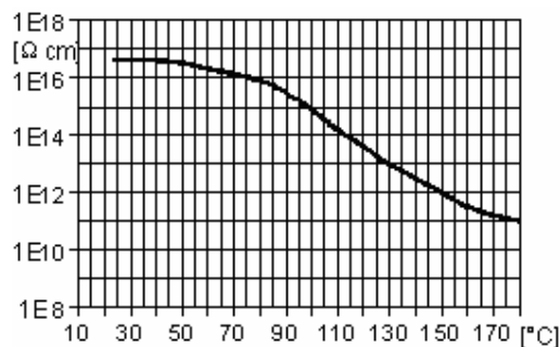
Fig.6.2.3: Volume resistivity ( \rho ) in function of temperature (system 3) (measurement voltage: 1000 V / IEC 93 / DIN 53482)
